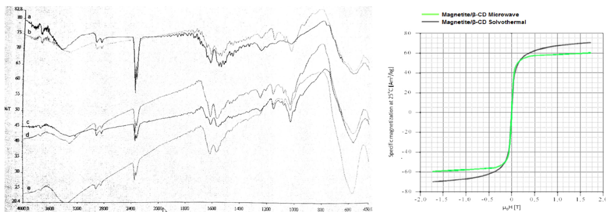
Fig.1. Left: FTIR characterization results for nanoparticles prepared via (a), (e) microwave assisted co-precipitation and (b), (c), (d) solvothermal method with stirring and ultrasound dispersion. Right: VSM characterization results for both types of nanoparticles
