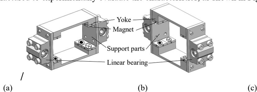
Fig. 1 Basic constructions: (a) overall; (b) X mover; (c) Y mover
