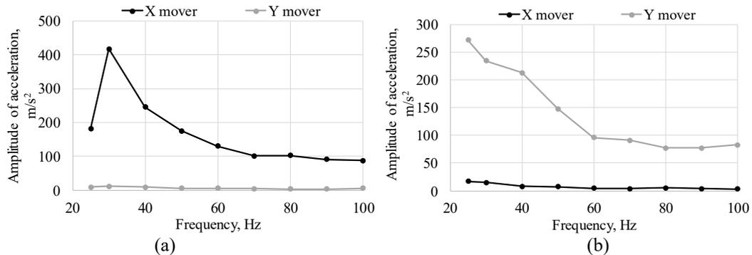
Fig. 3 Measured acceleration: (a) current is applied to X coil; (b) current is applied to Y coil
