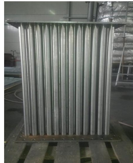
Fig.2. Heat exchanger built with plain tubes
