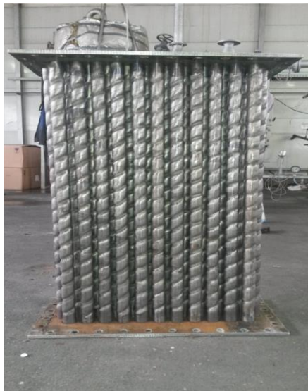
Fig.1 Heat exchanger built with explosively formed tubes
